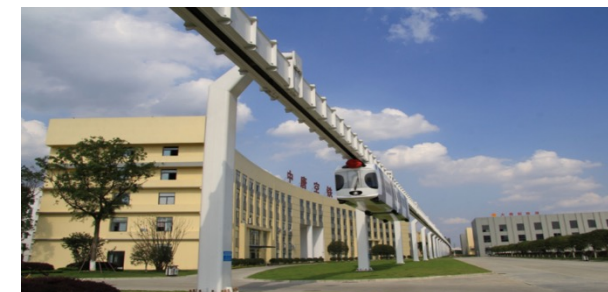
The second generation half-rigid half- flexible suspended monorail system
