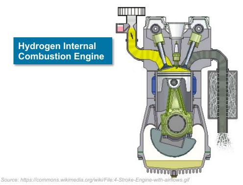
Conventional 4-stroke internal combustion engine technology
